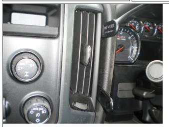
1. Press the thin end of the enclosed gap openers into the gap between the air vent frame and the padded part of the dashboard, to widen the gap.
