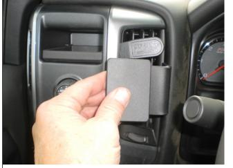
3. Press the thin end of one gap opener into the gap between the air vent frame and the frame surrounding the panel, to widen the gap. Press the thin end on the left side of the ProClip into the gap below the gap opener. Pull out the gap opener.
