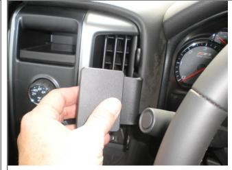
2. Peel off the cover of adhesive tape on the ProClip. Note: The adhesive tape does not leave any marks or damage the dashboard, and is easy to remove. Place the ProClip in your hand so the ProClip label (sticker) is in an upright position, or if vertically positioned; the P in ProClip is at the top.
